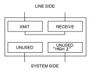
CHANNEL LOOP BACK is selected by setting to '1' the bit CLB in LSCR register.
