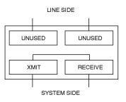
REMOTE LOOP BACK is programmed by setting to '1' the bit RLB in LSCR register.
